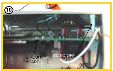
Gently pull the circuit board from the right stand-off. Pull circuit board out from the chassis just enough to access fuses.
