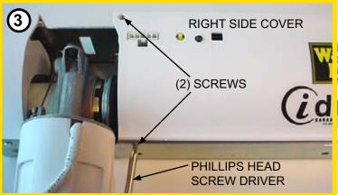
Using a phillips head screwdriver, remove the two screws from the right side cover.
