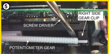
Gently remove the Potentiometer gear from the right side gear clip.
