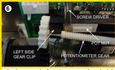
Gently remove the Potentiometer gear from the left side gear clip.
