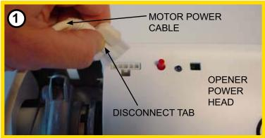
Carefully push the disconnect tab on the bottom of power cable and remove motor power cable from opener power head.
