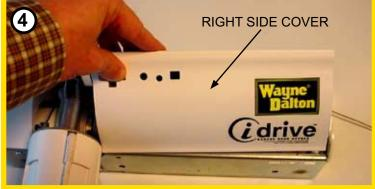
Remove right side cover from the opener to expose electronics and wiring.
