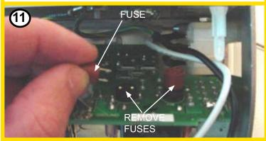
Locate the (2) fuses and remove.
