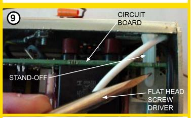
Using a flat head screwdriver, push the right stand-off locking tab to release the circuit board.
