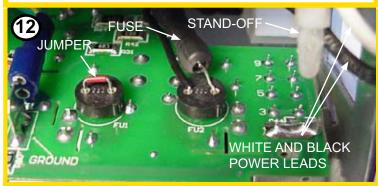
Insert fuse into FU2 fuse socket and bend it over as shown. The fuse must be angled to clear the power inlet wires when board is re-inserted. Insert jumper into FU1 fuse socket as shown.
