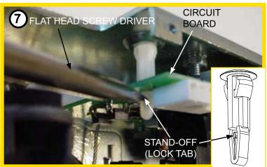
Using a flat head screwdriver, push the left stand-off locking tab to release the circuit board.
