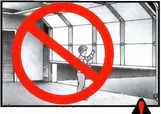
Teach children to keep their hands and fingers clear of section joints, hinges, track, springs, and other door parts. Contact with a moving door or its hardware could cause serious injury. These injuries can also happen with garage doors that don't have automatic openers.
