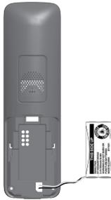
1. Plug the battery connector securely into the socket inside the handset battery compartment, matching the color-coded label.
