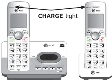
4. Charge the handset by placing it face up in the telephone base or charger. The **CHARGE** light is on when charging.
